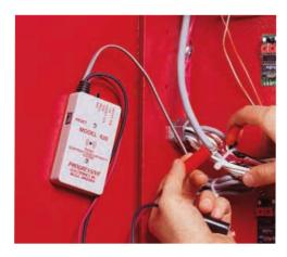
Designed for the security and alarm industry, the PE620 Loop Verifier offers convenience, ease of use, and true performance. As a continuity tester, the PE620 can be connected to a Normally Open or Normally Closed loop pair and provides a distinct audible tone when the alarm condition occurs.
