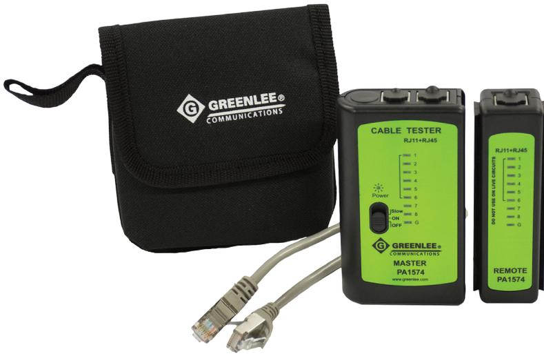
The PA1574 from Greenlee Communications tests the continuity of 8-way (RJ45) data and network and 6-way (RJ11) telephone patch cords and installed cable runs. It maps the cable, line by line and identifies good connections, opens, shorts and crosses. Includes patch cords, 9V battery and carrying pouch.
