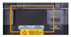
② Disengage the universal adapter first when the photo diode (receiver) on optical power meter is contaminated.
