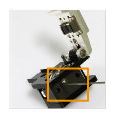
② Insert a wrench into the hole at the bottom of the cleaver and loosen the Setscrew of the slider a little bit (about 2 turns).
