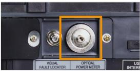
③ Subsequently, clean the photo diode with an alcohol cotton swab and then with alcohol-free one again.
