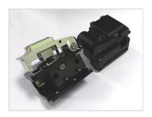
③ Open the cover and push the slider forward. When the slider is fixed, loosen the set screw a little bit (about 2 turns) with a hexagon wrench.
