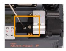
② Remove the Chip-Box using a hexagonal wrench as in the figure. (Optional)
