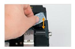
② When the cleaner is drained, open the cap and refill the cleaner.
