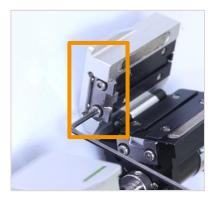
② Place new blade in the reverse manner of removing. (Two blades as a pair at top and bottom) For the perfect setting and fine stripping, there should be no cracks when the top and bottom blades make contact.
