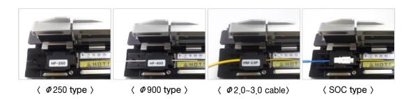
3 Mount the holder with the fiber onto the slider and close slide cover.
