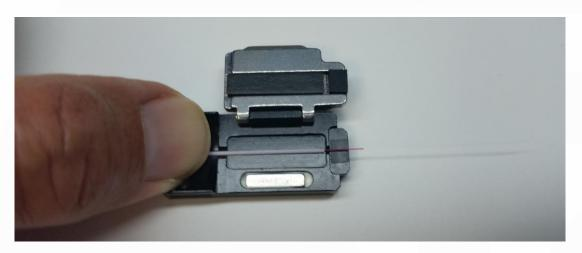
The 900 micron loose tube must not be held by the small fiber clamp on the far right hand side but only with the larger main clamp.
