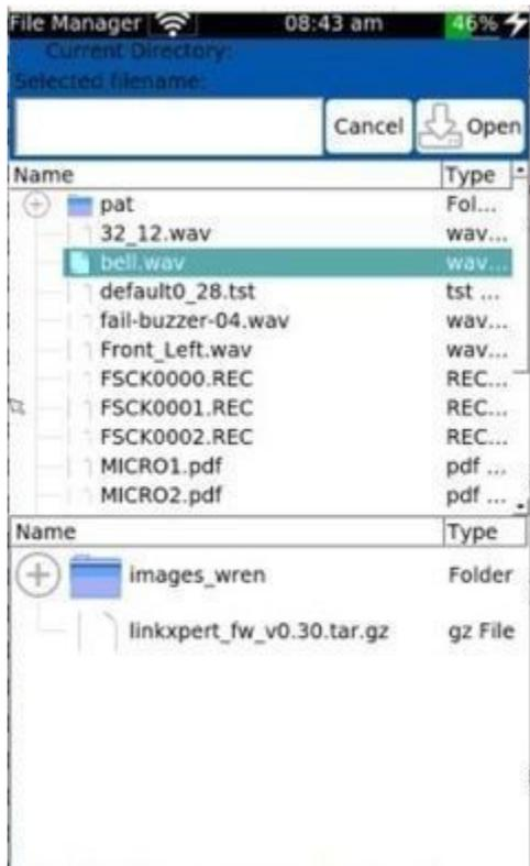
The upper area of the screen now shows the system memory of the LinkXpert, the lower area shows the memory content of the USB stick.
