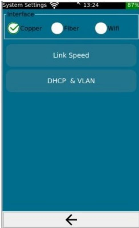
The network settings of LinkXpert are global settings and are independent of the test profile used. Settings are made separately for each interface.
