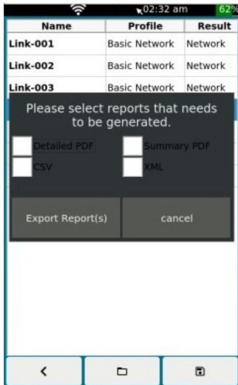
Reports in PDF, XML or CSV format can be created directly on the device.
