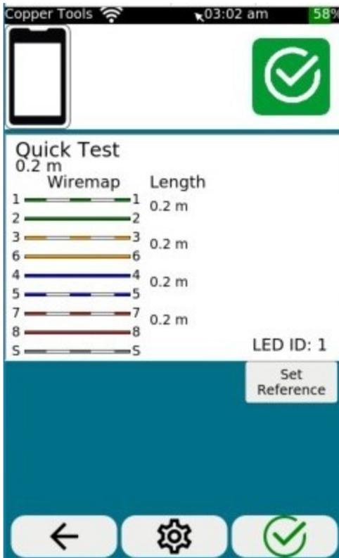
The wiring diagram is given per pin, the length per pair. The shortest length is shown in the report as link length.
