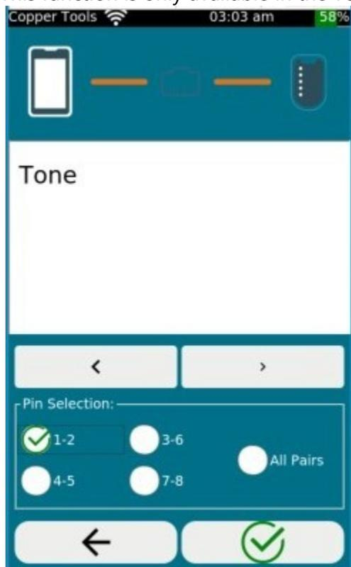
The built-in tone generator is compatible with analog cable locators such as Softing CP15. This menu is only accessible in the Tools module.
