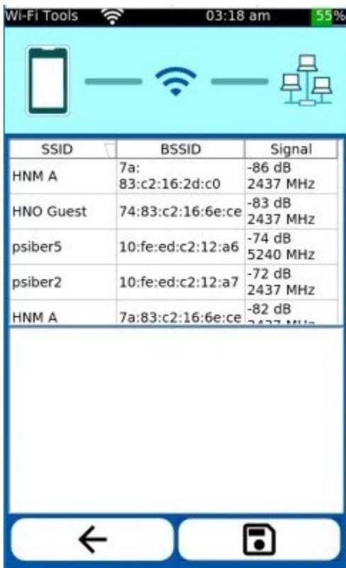
In the **WiFi Scan** test, LinkXpert M3 scans the 2.4 and 5 GHz bands for access points and lists the access points.
