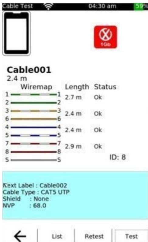
In the wiring test module, the device displays the wiring diagram with lengths.
