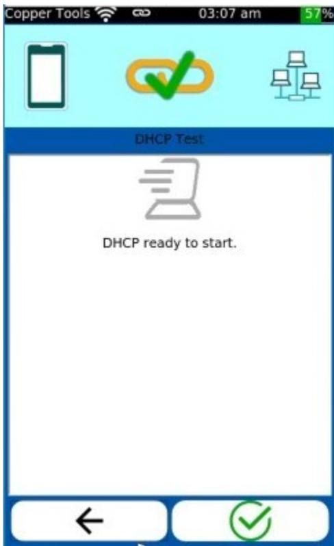
In the **DHCP Test**, LinkXpert checks whether the device can be assigned an IP address by the network and whether other information such as DNS server address and address range is transmitted.
