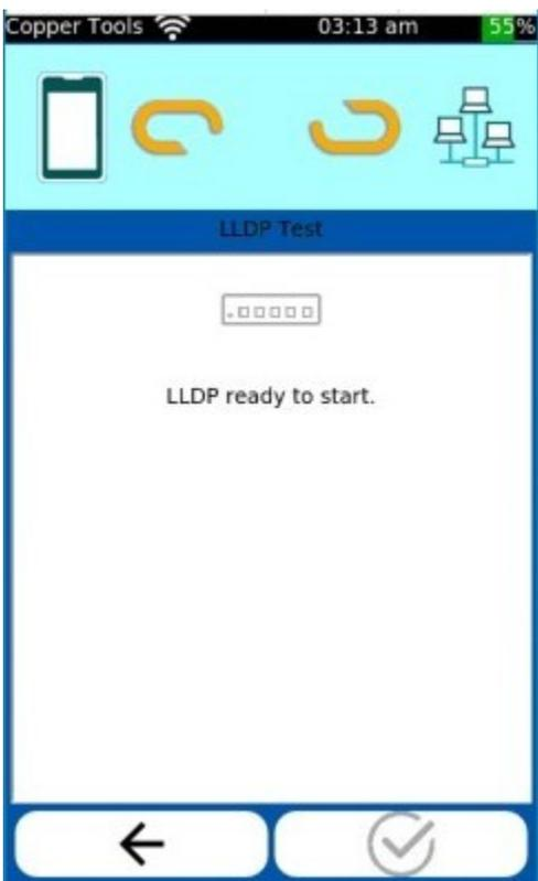
In the **LLDP** test LinkXpert lists LLDP responses of the connected switch.
