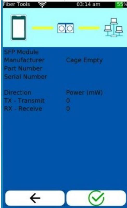
In the **TX/RX** the transmit (TX for Transmit) and receive values (RX for Receive) of the SFP module as well as information about the SFP module are read out.
