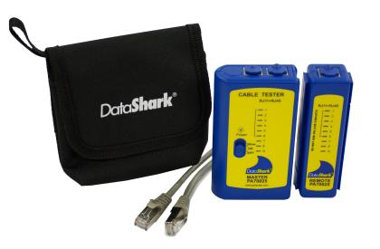
The Data Shark Cable Tester from Greenlee Communications tests the continuity of 8-way (RJ45) data and network and 6-way (RJ11) telephone patch cords and installed cable runs. It maps the cable, line by line and identifies good connections, opens, shorts and crosses. Includes patch cords, 9V battery and carrying pouch.
