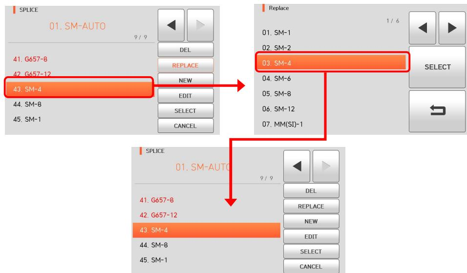
The splice mode from No.1 to No.42 can't be replaced.
