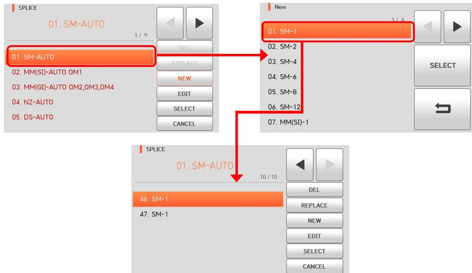
The splice mode from No.1 to No.42 can't be added.
