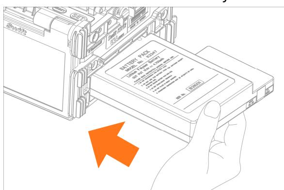
Insert the battery into the battery groove until it clicks.
