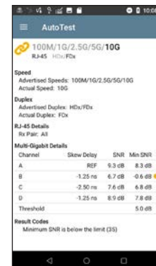
Cabling SNR measurement validates Multi-Gig links
