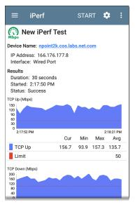
Test characteristics and status are displayed at the top of the iPerf results screen while the lower part of the screen displays a real time graph of the TCP or UDP Upload and/or Download speed. **Device Name**: Hostname or address of the iPerf server/Test Accessory
