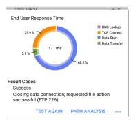
**End User Response Time graph**: Pie chart of the times for each phase of the test (DNS, Lookup, TCP Connect, Data Start, and Data Transfer)
