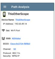
The example image above shows the SSID, Channel, and other Wi-Fi information the EtherScope can display after running a Path Analysis over Wi-Fi.
