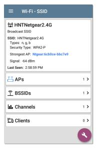
In addition to the Signal and Security Type, the SSID Details displays the AP on the network with the strongest signal, 802.11 Types that the APs in the network support, and the time the EtherScope last detected activity on the network (Last Seen).
