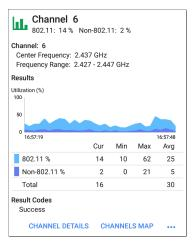
The Channel Test results screen indicates the Center Frequency and Frequency Range of the connected channel along with a real-time Utilization graph.
