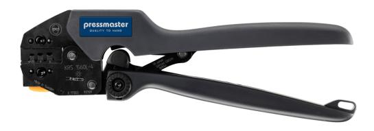
KRS-1560L-4 is a crimping tool for Solar connectors like MC4<sup>™</sup> and similar connectors, Ø 4 mm/.157", with openbarrel conductor crimp 1.5 - 2.5, 4.0, 6.0 mm<sup>2</sup>/AWG 16 - 14, 12, 10. This tool also exist in versions for MC3™ and SOLARLOK™ connectors. (MC3™ and MC4™ are trademarks owned by Multi-Holding AG, Switzerland. SOLARLOK™ is a trademark owned by TE Connectivity, USA)
