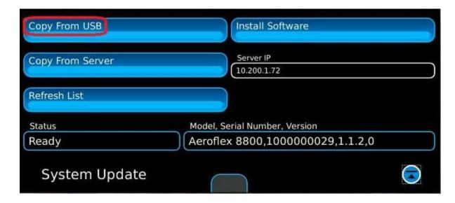
7. After the status field shows "Files are ready to install", press Install Software. At this point it is safe to remove the USB flash drive.
