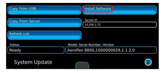
8. The screen will go black for a moment, then a progress bar will appear showing the installation progress. After the update is complete, you will be prompted to cycle power on the unit. The update is complete.
