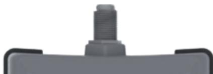
**Figure 6.** F-Connector on Main Tester
