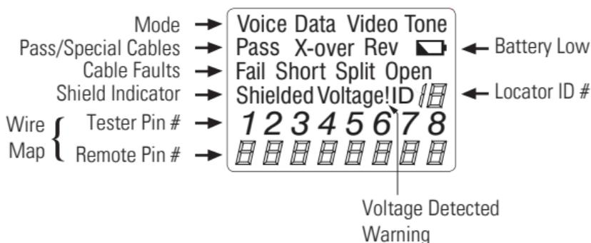
Figure 2. LCD Display Screen
