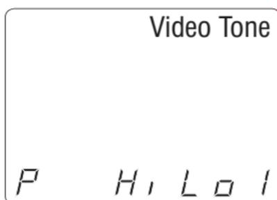
**Figure 12.** Video Cable Test with Pin Selected
