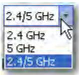
Changing operating frequency is just like physically changing the wireless network card. AirMagnet WiFi Analyzer will empty all the packets captured in the buffer and then start capturing data using the new operating frequency. Any change in operating frequency is reflected in other parts of the UI that are affected. If you are on a screen other than the Start screen, selecting another band will take you directly to the Start screen.
