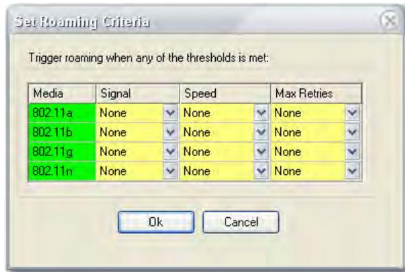
2. Click the down arrows to adjust the **Signal**, **Speed**, and **Max Retries** values for the 802.11 protocols on your laptop computer when it enters roaming state.
