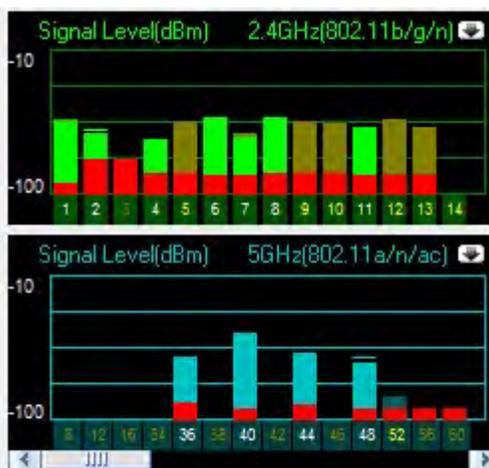
This part of the screen consists of two sections: the upper part shows the 2.4-GHz band and all available 802.11b/g/n channels while the lower part the 5-GHz band and all available 802.11a/n/ac channels.
