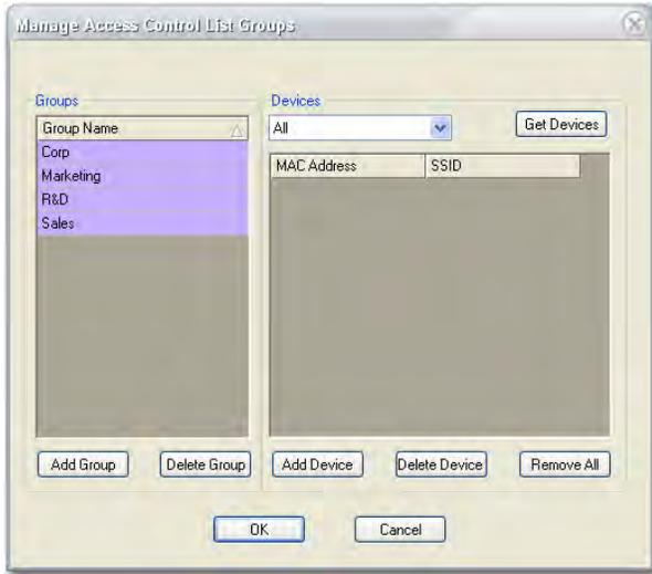
**Note:** Corp is the default ACL group that contains all the devices AirMagnet WiFi Analyzer has discovered on your network. You need to create new ACL groups and assign the devices to different groups. Refer to the table below for descriptions of the buttons in the Manage Access Control List dialog.
