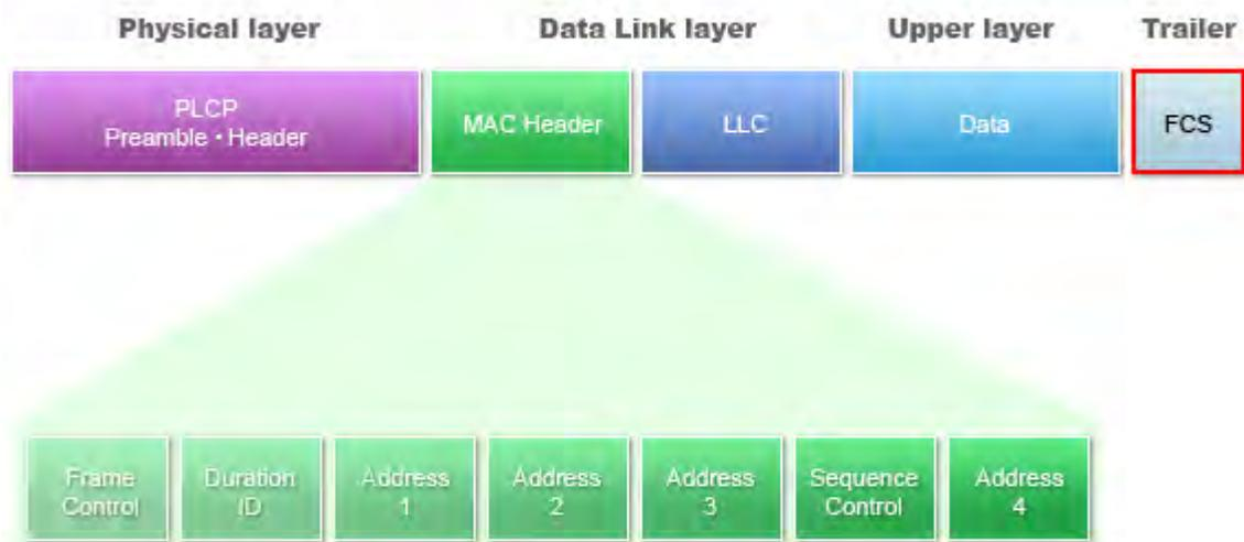
**IEEE 802.11 Frame Includes Checksum in PLCP and FCS for Frame Header and Frame Body Respectively**
