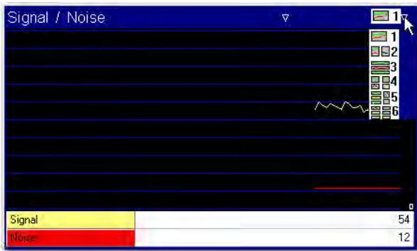
**Note:** When a specific device (that is, AP, station, ad hoc) is selected, the graph shows data about the selected device only; when a channel is selected, then the graph will display data for the entire channel.
