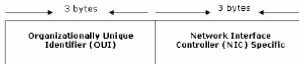
By default, MAC addresses of all existing wireless networking devices are already mapped with the names of their respective vendors. AirMagnet WiFi Analyzer's Start screen reflects such mappings. AirMagnet periodically updates the MAC-vendor name mappings used in its products as new hardware devices come to the market. The *LANCardVendorsFile.txt* file is intended solely to help users who want to create the MAC-vendor name mappings on their own, without waiting for an AirMagnet's update.
