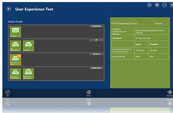
Detailed metrics such as Round Trip Time (average and max), HTTP Download Throughput, and number of interruptions that occurred during execution of the video test can be obtained.
