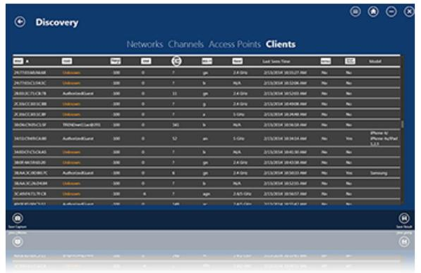
Note: \*Proxim Orinoco 8494 802.11a/b/g/n USB adapter (US/WD/JP versions) is required for detecting clients and SNR/channel utilization information.
