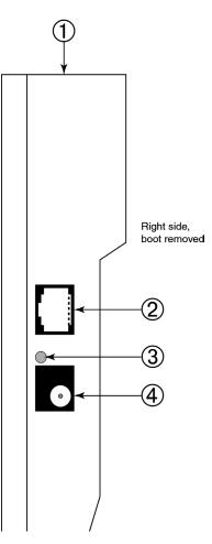
4. DC input receptacle: The power transformer/NiMH battery charger is connected to this receptacle.
