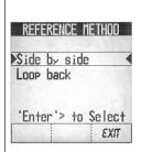
From the Autotest Main screen, press the REF softkey. The Reference Method screen will be displayed. Use the UP/DOWN arrow keys to highlight ➤ SIDE BY SIDE or ➤ LOOP BACK
