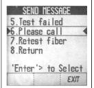
The 525-30 has eight stored messages that can be sent between units when performing Insertion Loss testing. These messages are pre-programmed and cannot be modified by the user -
