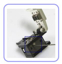
3 Turn the markings on the blade counter clock wise one by one with a cotton swab.
