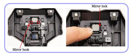
3 Insert a new mirror into the mirror lock and assemble the parts in reverse manner of disassembling.
