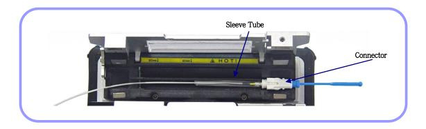
Activate the heater after placing the fiber. Cooling fan is run to cool the tube 20 seconds after heater activation.
