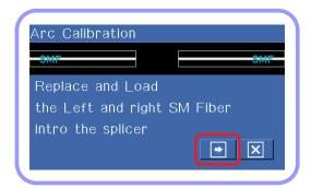
Discharge is carried out after arranging the fibers and the amount of discharge is adjusted according to the discharge condition.
