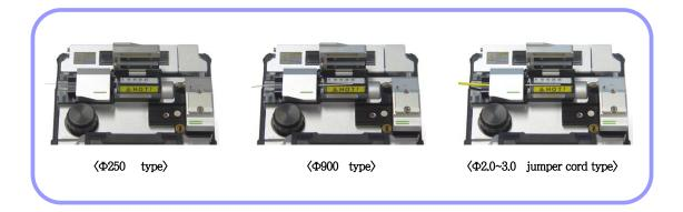
4 Once the thermal stripper cover is closed, the fiber is heated up for a predefined time and the coating is stripped by moving the slider.
