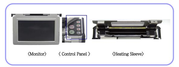
2 Set the sleeve tube to the area of arc-fused fiber that needs to be reinforced and place the fiber inside the heater.
