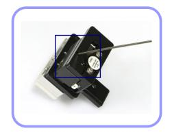
3 Insert the wrench bolt into the cam pin and pull it with tweezers and detach the slider.
