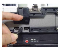
The battery pack includes the protection circuit so that over discharge and over charge can be prevented. The supply of power stops once the protection circuit is activated. In order to deactivate the protection circuit and resume feeding power, wait about 10 seconds and connect the DC plug to the DC jack of the battery pack and the AC cord of the charger to a wall outlet.
