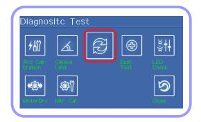
1 The self-diagnosis can start by pressing "ENTER" or tapping the screen after removing fibers from the device. See the table below.
