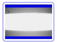
The splice loss value is measured after completing arc fusion and displayed on the screen. The loss value is affected by error elements. And, these elements also influence the estimation and computation of the value. The computation of the loss value is based on such clear measurement factors as MFD.
