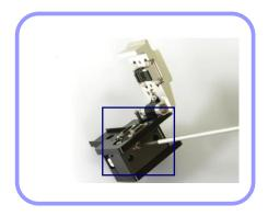
When the blade reaches required position, tighten the set-screw of the slider. Thoroughly and accurately set the height using a gauge because the height directly effects the cleave quality of fiber.
