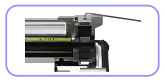
(2) The Choice of Heater Block / Lever Block by fiber type
