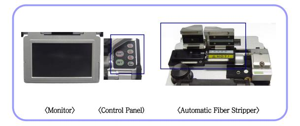
2 Place fiber into the holder as shown below pictures. The minimum stripping length should be longer than 18mm.
