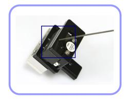
2 Adjust the blade height by turning Cam Pin with a flat-head screwdriver.
