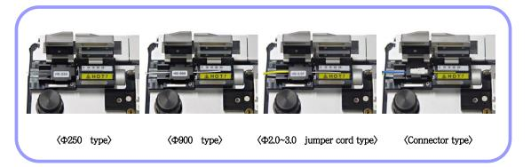
3 Mount the holder containing the fiber onto the slider and close slide cover.
