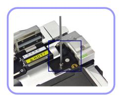
2 Open the cover and push the slider forward. When the slider is fixed, loosen the set screw a little bit (about 2 turns) with a hexagon wrench.
