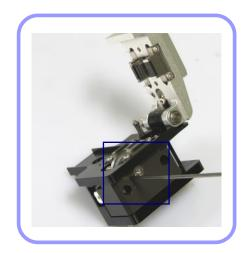
2 Insert a wrench into the hole at the bottom of the cleaver and loosen the set screw of the slider a little bit (about 2 turns).
