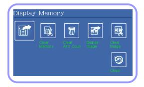
It can be selected using left and right keys and "ENTER" or tapping the screen.
