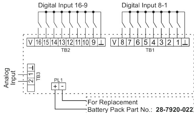
Fig. 5: Wiring diagram
