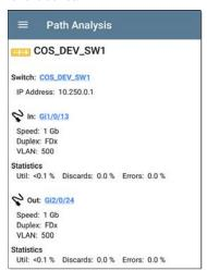
A Layer 2 Details screen displays the device name and IP address at the top.
