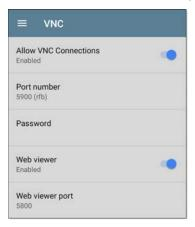
Allow VNC Connections: Touch the toggle button to enable or disable remote connections from VNC clients.
