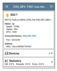
The Interface Details screen contains a description of the interface and information about its Status, Connected Device and Port, and Address.
