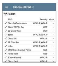
On the SSIDs screen, each SSID is shown with its Security type(s) and any VLANs. SSIDs with a checkmark to the left are enabled, and those with an X are disabled.
