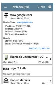
Like AutoTest, Path Analysis results are presented on cards. The top card shows the main test details, the second card shows information for the source device (your
